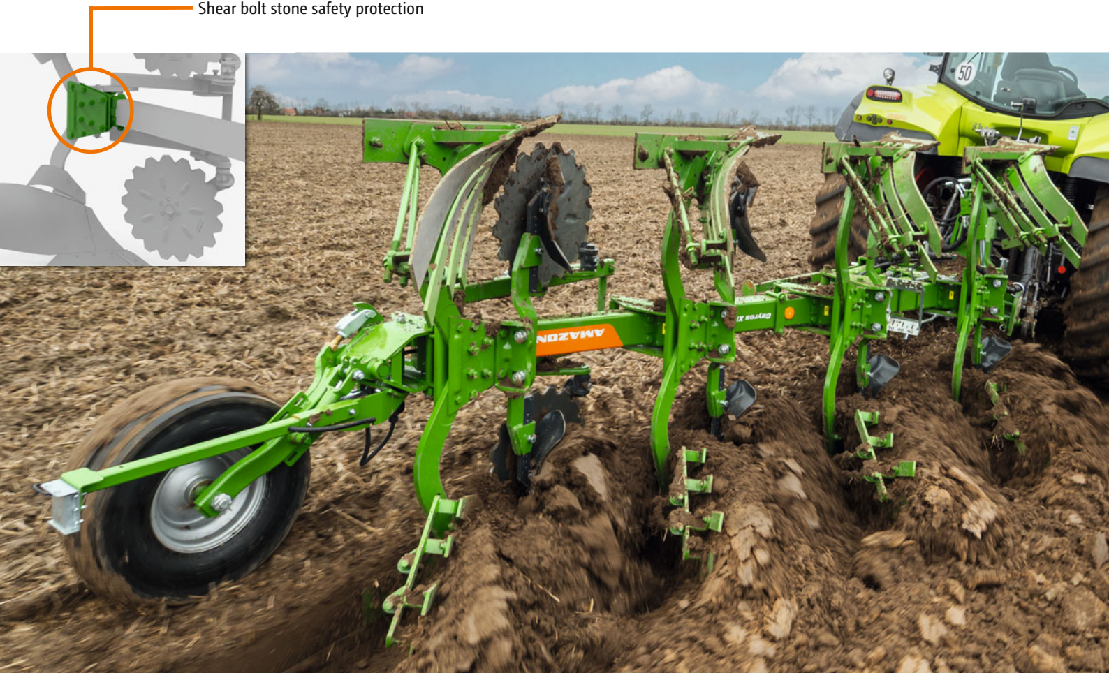
Shear bolt stone safety protection
