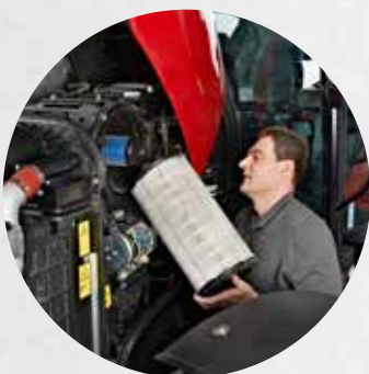
Continuous cleaning via a Piclon filter ensures that the filter only needs to be maintained when the corresponding warning lamp lights up.
